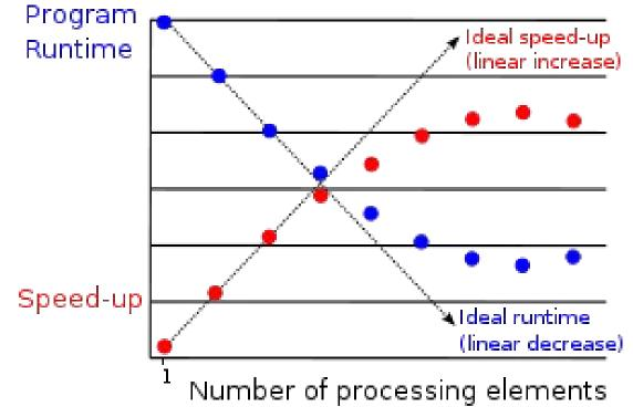
A diagram of the program runtime (shown in blue) and program speed-up (shown in red) of a real-world program with sub-optimal parallelization. The dashed lines indicate optimal parallelization– linear increase in speedup and linear decrease in program runtime. Not: the runtime actually increases with more processors (and the speed-up likewise decreases) -> this is parallel slowdown.
