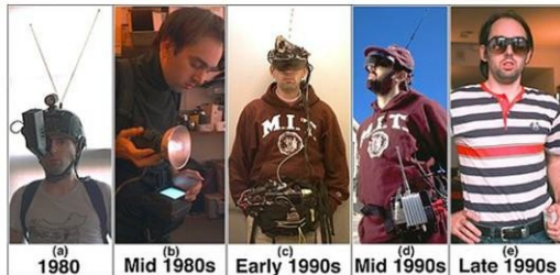
Evolution of Steve Mann's WearComp wearable computer from backpack to the current covert system
